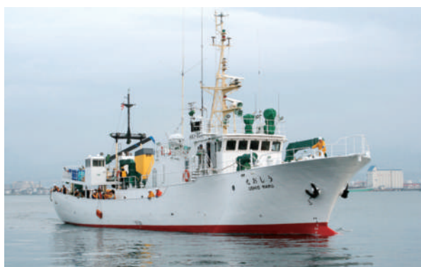
Constructed: September 28, 1992 / GT: 179 tons / Length: 39.39m / Crew capacity: 33 / Annual number of days at sea: 170 / Voyage waters: Around Hokkaido
