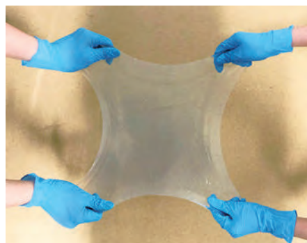
Novel gel-like adhesive obtained in this study, which has high strength and elasticity
