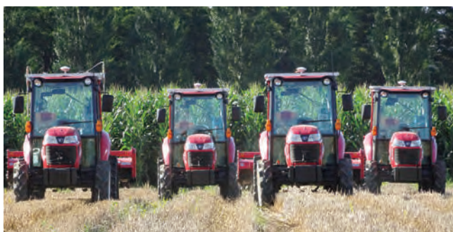
Collaborative tillage work of four unmanned tractors. Collaborative work of multiple tractors is a system inspired by the ideas of farmers (left). The farms attract many visitors from Japan and overseas (right).
