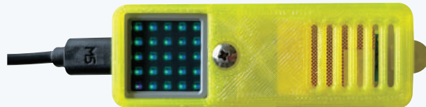
Prototype CO 2 densitometer with warning display function
