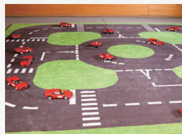
Experiment on self-driving cars that yield the right-of-way to each other using the Deep Q-Network algorithm conducted by the Harmonious Systems Engineering Laboratory
